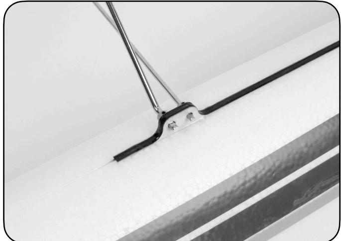
1. Secure the set screws to the flat spot closest to the middle of all of the struts and spreaders. Pay special attention to the size of the strut and inside diameter of the wheel collars. Use blue thread lock to secure the set screws in place.
